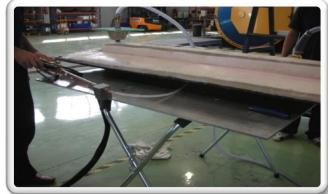
RTM – Resin Transfer Moulding
